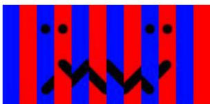
Step 2: Interlace them (cut the two images into strips and join them together so the strips from the first image alternate with the strips from the second image).
